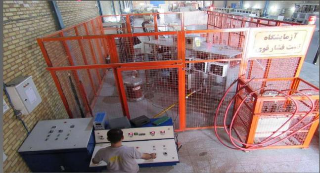
Impulse test :Apply voltage up to 100kv at specified time
