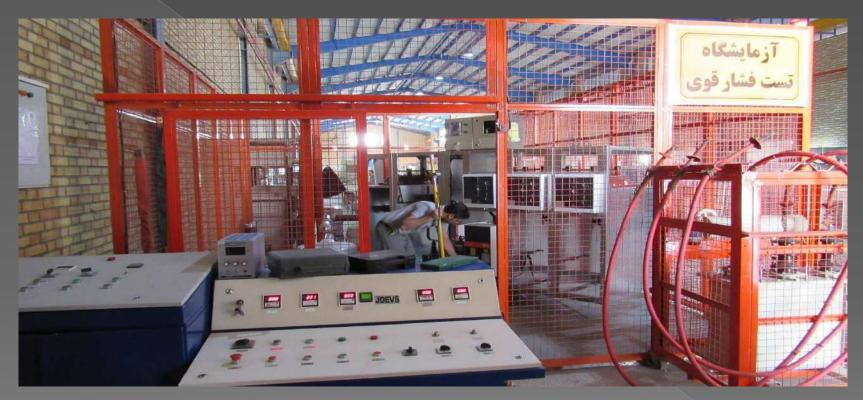
Power frequency test: Apply voltage 50-100 KV for one minute
