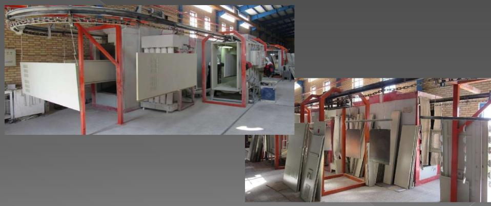
Electrostatic color that blows the powder to the product and enters the furnace
