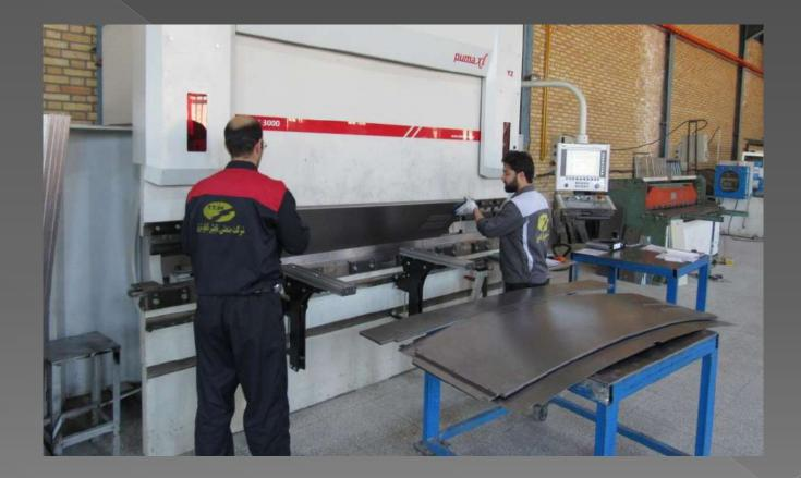
Bending machine capable of bending up to 3m wide
