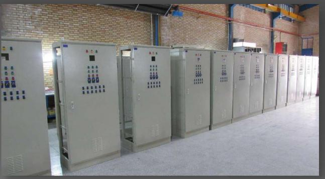
Protecting these boards against objects larger than one millimeter
